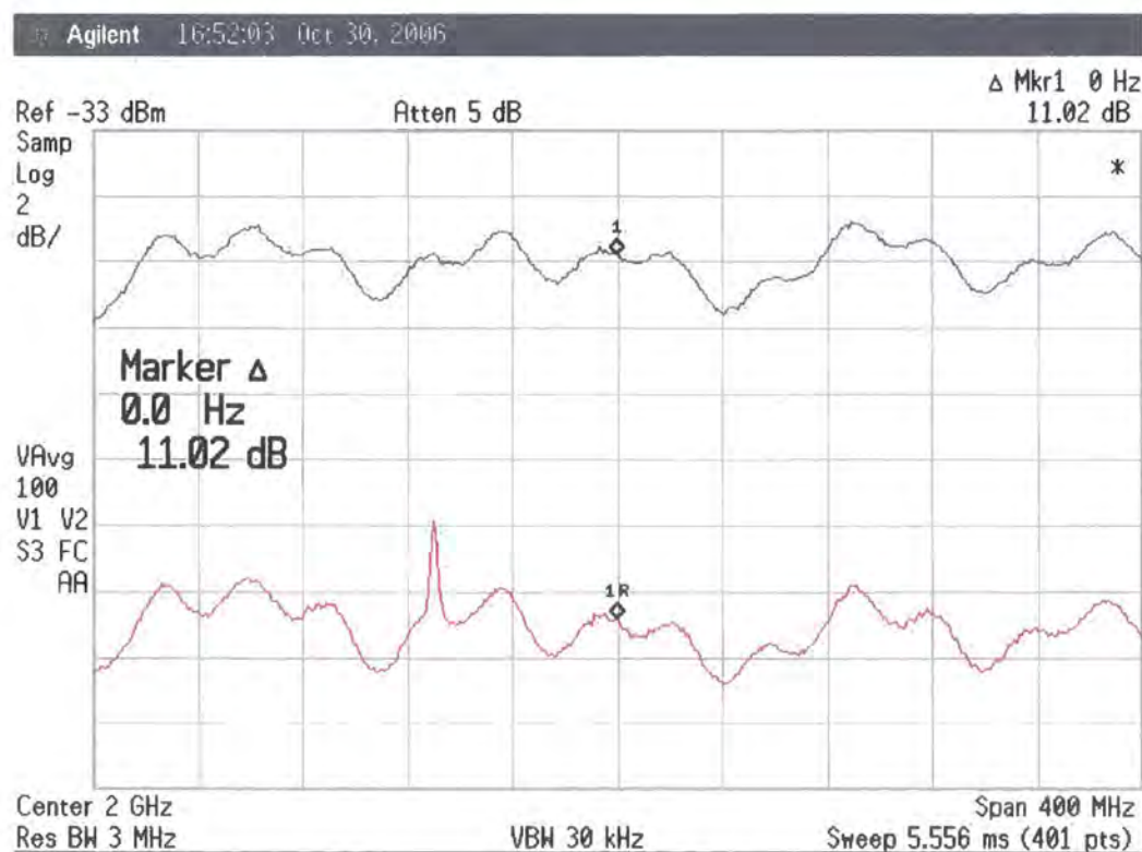
Figure 5.14 “y-factor” measurement of the 2.5 GHz down-converter
