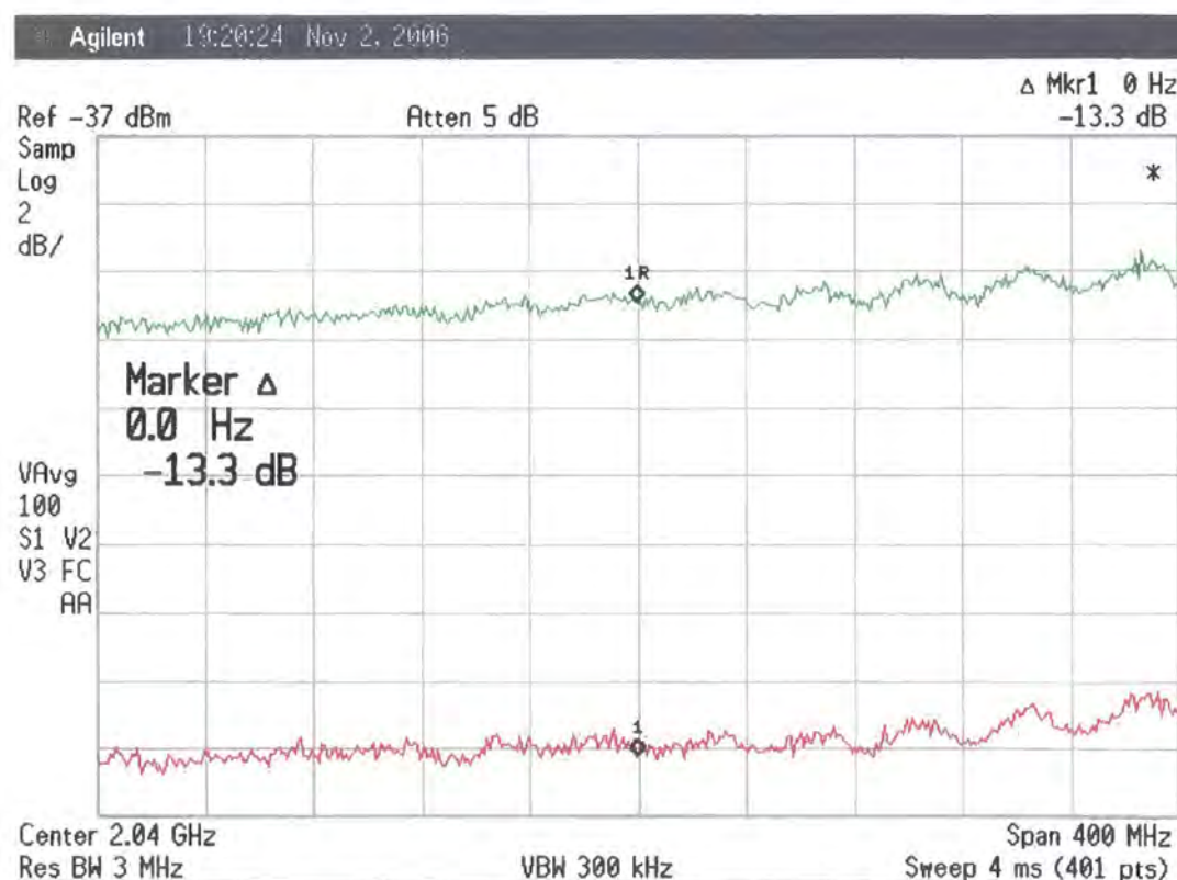
Figure 5.18 “y-factor” measurement of channel 2 of the four-channel converter
