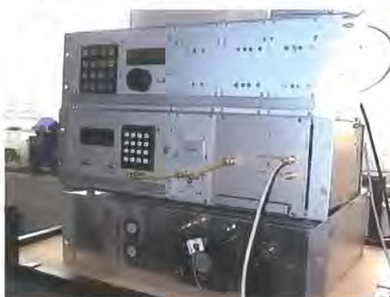
Figure 3. Complete multi-band sounder transmitter
