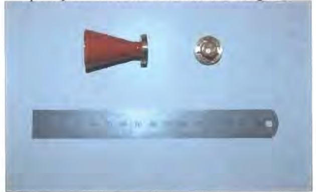
Figure 5. Horn antennas (20 dBi on left, 10 dBi on right).
