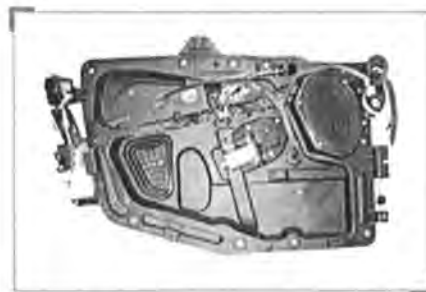
Figure 5.3: Door carrier [Faurecia doors]
