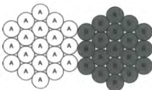
Figure 6.1a The two components exist as separate clusters of atoms combining as one nanoparticle.
