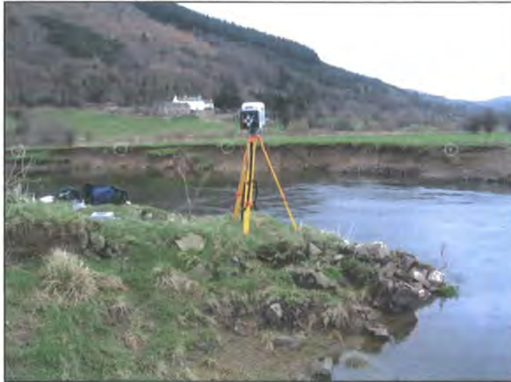
Figure 3.8: The laser scanner taking the first base scan of river bank 1, 13 th March 2007. The laser scanner is mounted on the yellow tripod. The scan targets used for referencing the scans are indicated (circled).
