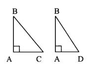
Thales stands on the tower at B with a stick and crosspiece to fix an angle. He fixes the stick upright and directs the crosspiece at the ship. He fixes the crosspiece at this angle, ABC. He creates triangle ABD, where D is the point on the shore determined by angle ABD being the same as ABC . The distance AD=AC, the distance of the ship from the shore.<sup>74</sup>
