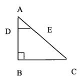
Thales stands on a tower at A with a right angle-shaped instrument. The small right angled triangle ADE has common angles to ABC, so the length of BC can be determined by DE by proportion. This does not require the use of much level ground. 71
