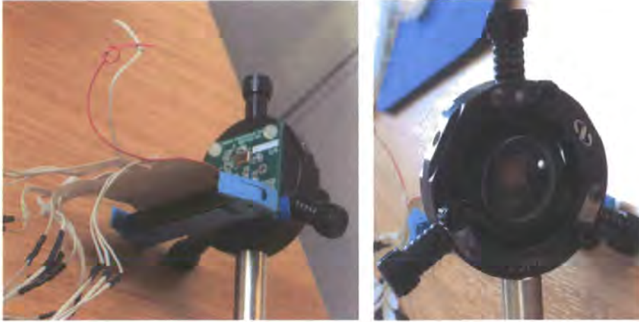
Figure 5.6: Wavefront sensor assembly - Photographs showing the LM9630 camera head-board screwed to the rear of a lens mount (left), which is clamping the microlens array held in a small barrel mount (right). In the later photograph the active area of the KAC9630 imager is visible through the microlens array.
