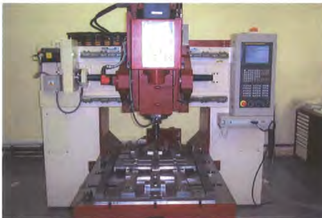
Figure 25 - Friction Stir welding Machine used for Trials
