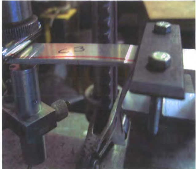
Figure 52 - TRIAL 3 C3 Extruded Bend Test Under Load
