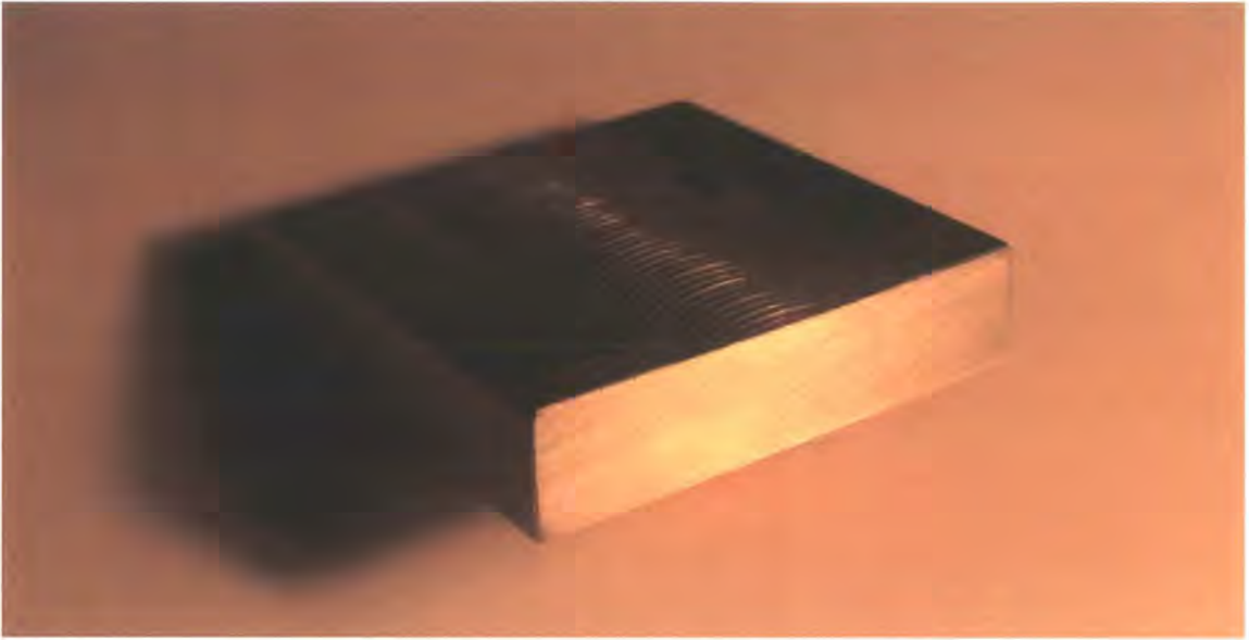
Figure 56 - Unflawed Section of C2 Weld from TRIAL 5
