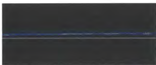
Figure 3-12 - As previous figure. Streak camera image in focus mode at high MCP gain. Shutters are open to detect the dispersed emission spectrum of an MeLPPP solution (greenish-yellow line). Compared to the grey horizontal line, the spectrum is detected with a slight tilt but still projected onto the photocathode area (blue) to its full horizontal extent.
