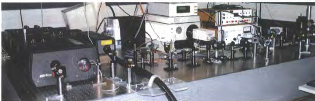
Figure 3-1 - Photograph of the laboratory with TCSPC and streak camera set up.
