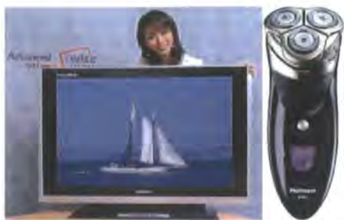
Figure 1-2 – In 2005 Samsung SDI presented its 40'' test PLED display with emphasis on blue emission. The Philips shaver model with monochrome PLED display is produced since 2002.
