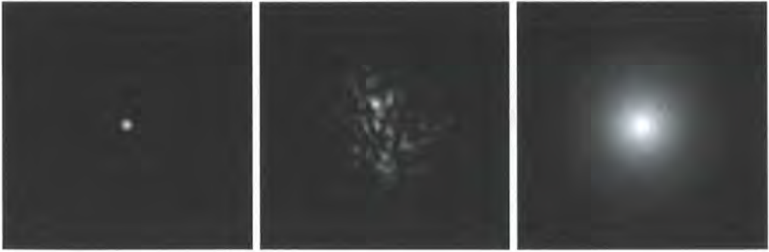
Figure 2.1: Example telescope PSFs. Left : diffraction limited, no aberrations (Airy disk); centre : large aperture, short exposure – note the “speckles”; right : large aperture, long exposure – speckles are averaged out. All 3 PSFs have the same image scale but the brightnesses are scaled independently. The aberrated PSFs were simulated with D/r_0 = 10 (see section 2.2 for definition of r_0 ).
