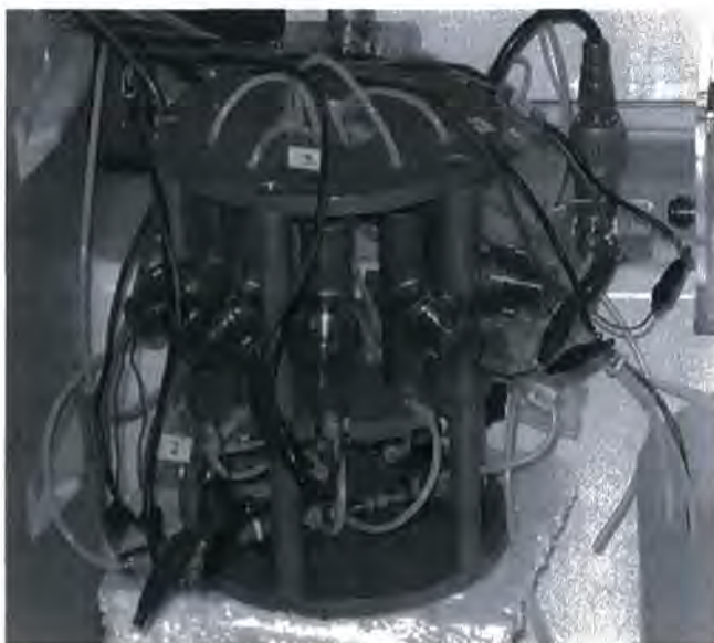
Figure 5.1: Five sample chambers with vapour lines connected
