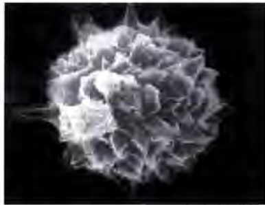
Figure 1.1: SEM image of a 1 micron diameter nickel particle found in QTC
