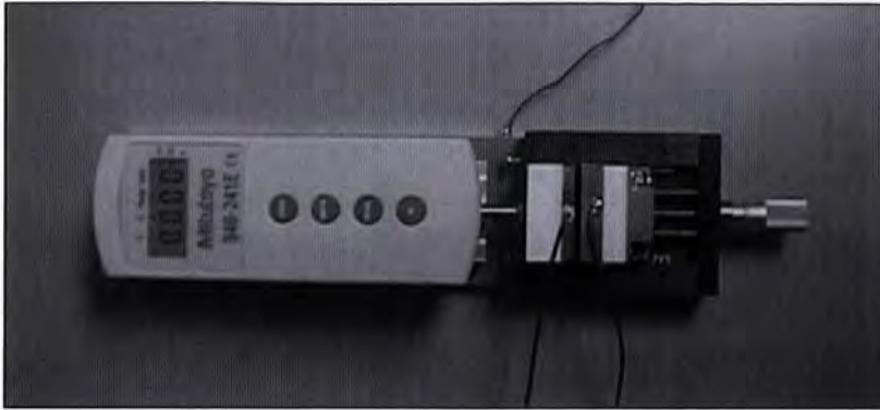
Figure 3.2: Setup to measure Resistance as a function of Force
