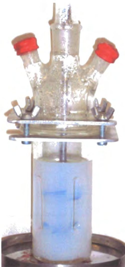
Figure 7.8: Latex particles from the emulsion copolymerisation of VBC and DVB in a baffled reactor vessel with twin bladed impellar.
