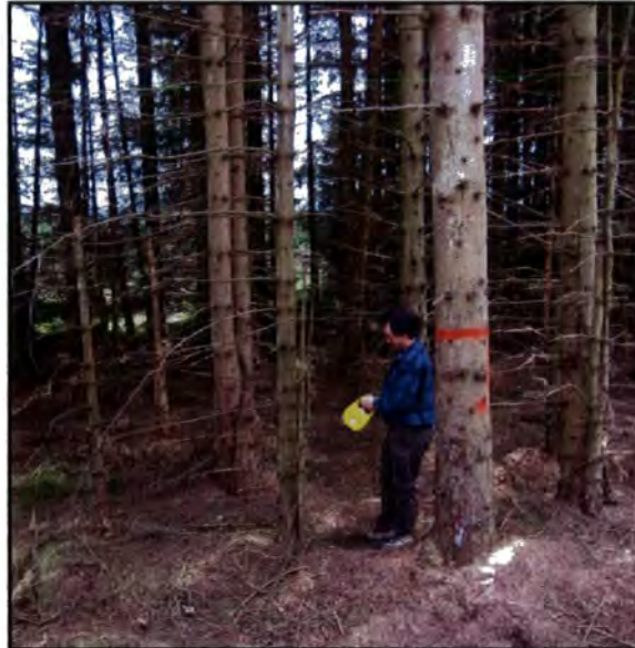
Figure 3.3 The trial area showing how the tree number and dbh was marked in orange. Field assistant using a tape measure as part of the technique of measuring tree height with a Suunto clinometer (Photo: A. Woodget 05.06.07).
