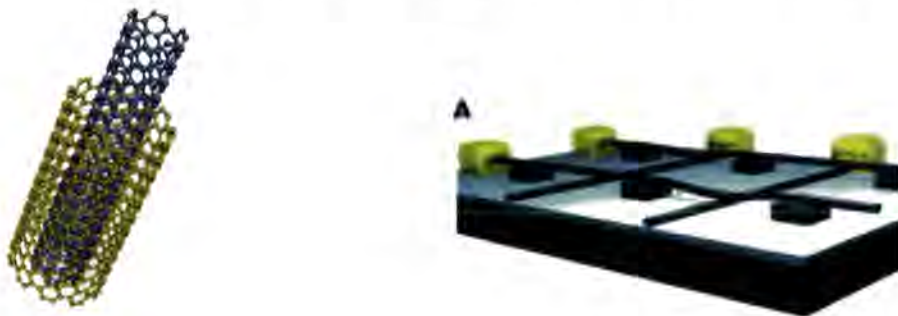
Fig. I.7 A double walled carbon nanotube 26 and a highly organised array of nanotubes. 27
