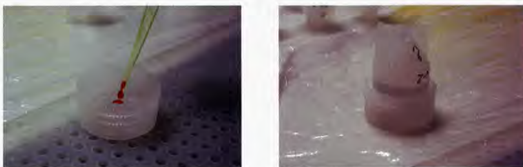
Fig 3.5 Shows the chromium oxide ( \text{Cr}_2\text{O}_3 ) being added to the 12N sulphuric acid ( \text{H}_2\text{SO}_4 ) droplet in the rocket vial lid. Fig. 3.6 Shows the rocket vial upside down and sealed with the hydrobromic acid (HBr) droplet in the bottom of the cone, and the chromium oxide and sulphuric acid in the lid.
