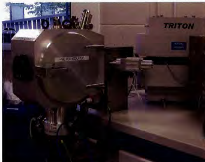
Fig. 3.11 Thermo Finnigan. Triton Mass Spectrometer (N-TIMS). The image shows the -ve ion source, used for Os analyses only.
