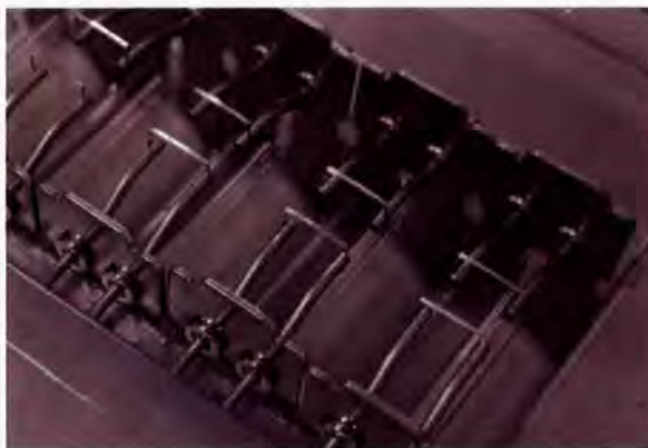
Fig. 3.10 Shows the filaments with their welded Pt ribbons, ready for the Os loading procedure.
