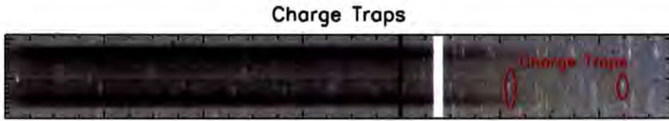
Figure 5.3: Examples of GMOS charge traps (white vertical streaks).
