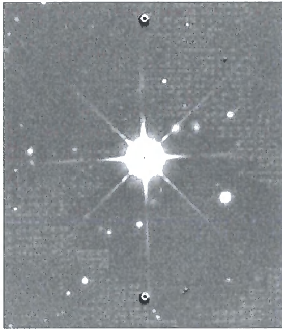
Figure 5.4: An example of cross-talk (doughnut shaped artifacts) in the detector read out direction caused by a bright star on a WFCAM image.
