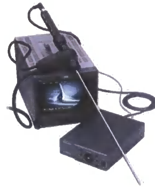
Figure 3.23. Camera Borescope with image rectifier
