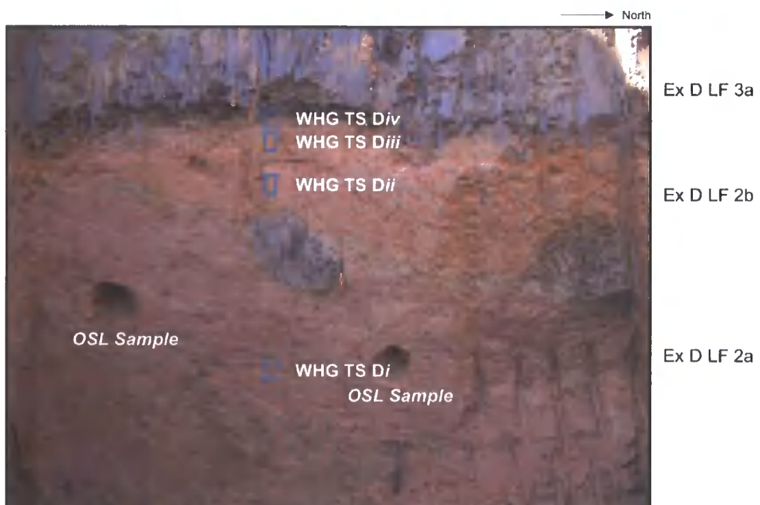
Figure 6.21: Location of thin section samples and OSL samples at Exposure D, Warren House Gill. Geological hammer is 32 cm long. Penknife is 19 cm long when extended.
