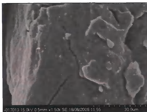
SEM images of Ni 2 TCNQ: Layered structure.
