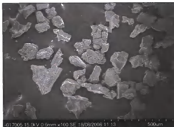
Figure 4.22: SEM images of \text{Ni}_2\text{TCNQ} illustrating the spread of particle size.
