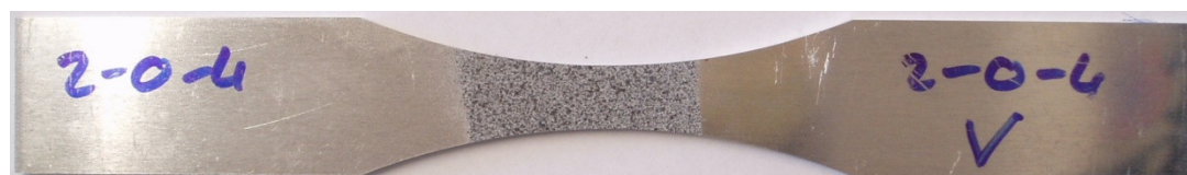
b) Specimen of varying cross-section, so plastic deformation restricted to small zone
