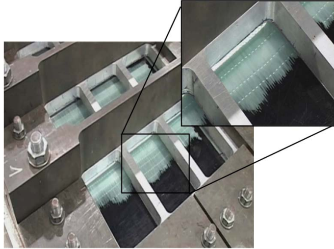
Figure 5.19 Resin flow front during RTM injection of glass composite with C100 filled suspension.
