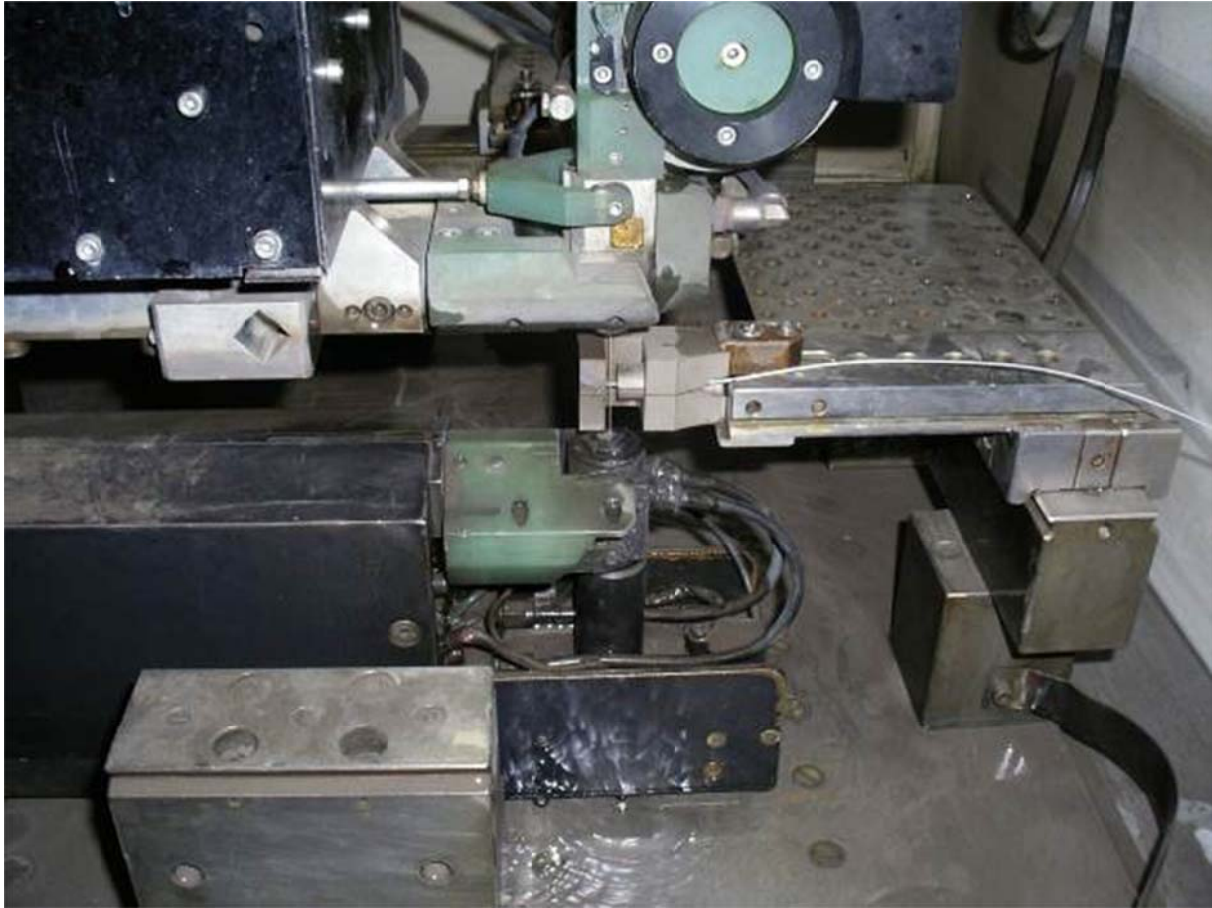
Figure 5-20 Clamping device mounted on Wire eroding EDM
