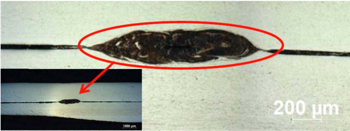
Figure 6-60 Cross-section through intermediate layers after explosion test (button)
