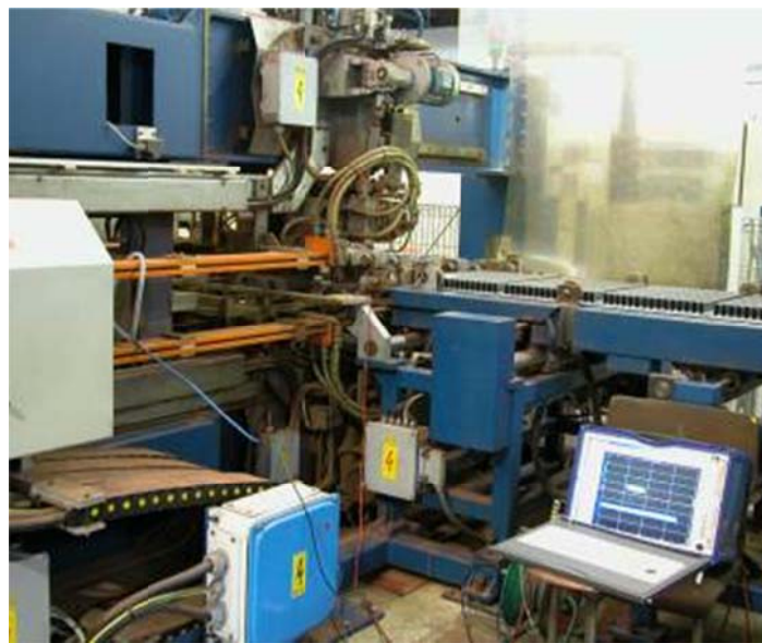
Figure 1-21 LEAS portal type roller seam welding machine on radiator production line (photo courtesy of Quinn Radiators)
