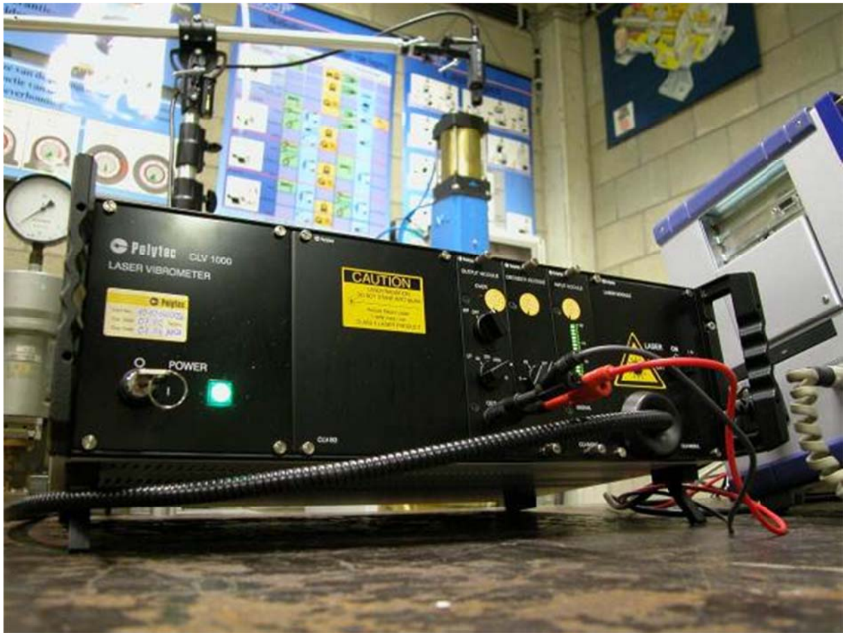
Figure 4-12 Polytec compact laser vibrometer
