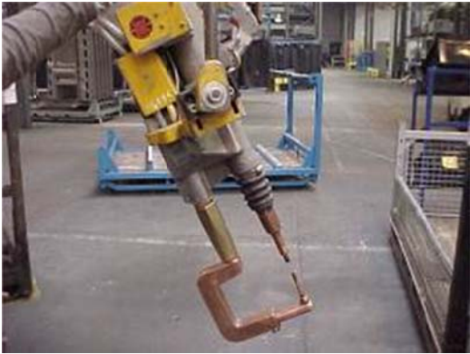
Figure 1-19 PW Portable C-type spot welding gun (photo courtesy of DAF trucks)
