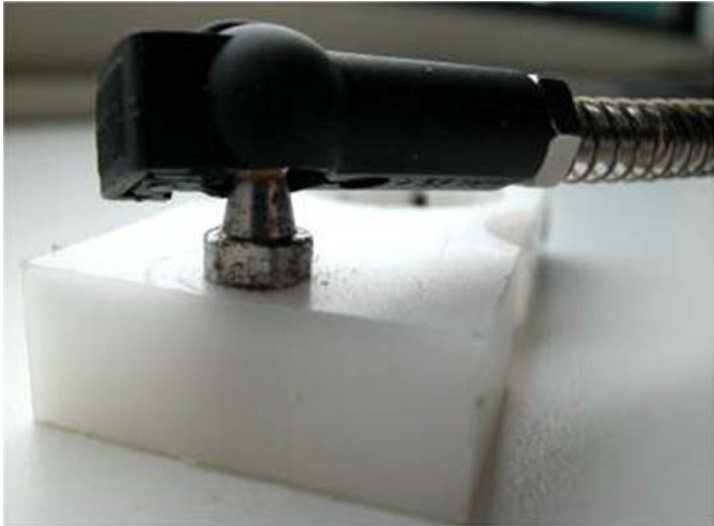
Figure 4-10 Plastic ball joint connected to upper end of LVDT
