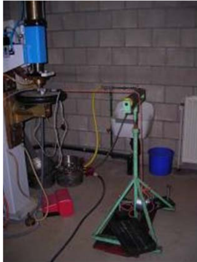
Figure 5-24 Application of lateral force on welding head
