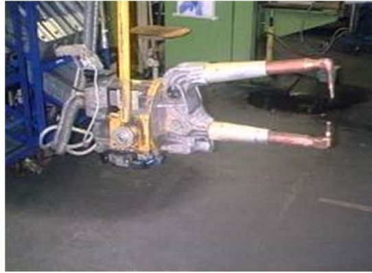
Figure 1-20 PW Portable Y-type spotwelding gun (photo courtesy of DAF trucks)
