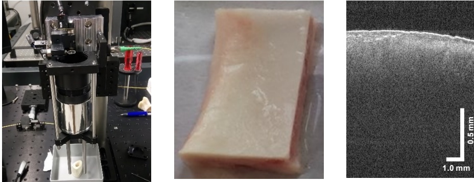
Figure 2. The custom developed Axsun swept source OCT system (left) used in this work, a porcine femur bone, sample (middle) and the raw OCT image example of the bone (right).
