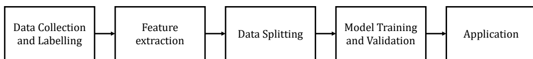
Figure 3.1: Common steps of building an automatic tissue characterization system in OCT. It starts with collecting images from an OCT device and manually labeling the tissue type of the corresponding image. It is followed by feature extraction to find unique characteristic features of a tissue embedded in the image. The extracted features are then split into training and validation datasets. A machine-learning model will be trained and validated before it is applied in clinical conditions. Additional testing datasets are usually used as a benchmark by which to evaluate the performance of the machine-learning model.
