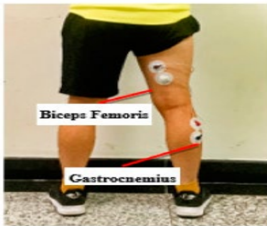
Fig. 2. Location of EMG sensors [13].
