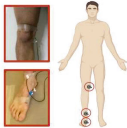
Fig. 3. Location of the triaxial accelerometers [14].
