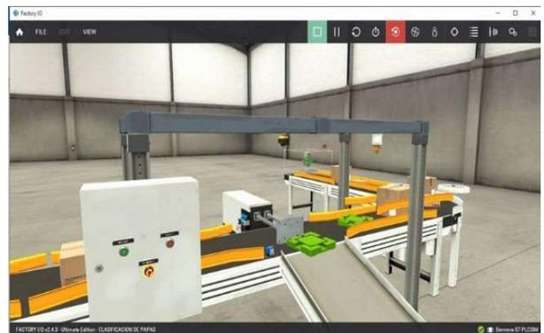
Fig. 8. Detection of green boxes (defective handles).
