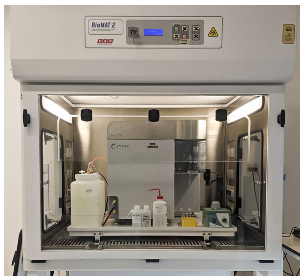
FIGURE 3 Example placement of a 3-laser benchtop analyzer inside a Class II Biological Safety Cabinet [Color figure can be viewed at wileyonlinelibrary.com ]
