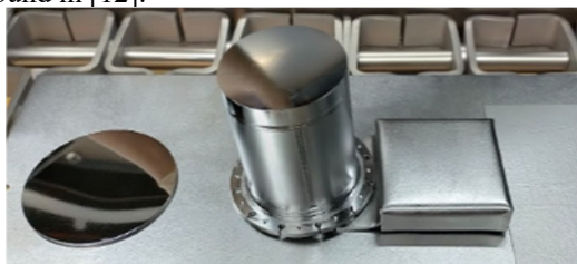
Figure 3: Nb bulk QPR sample after metallographic polishing prior to heat treatment @IJCLab.
