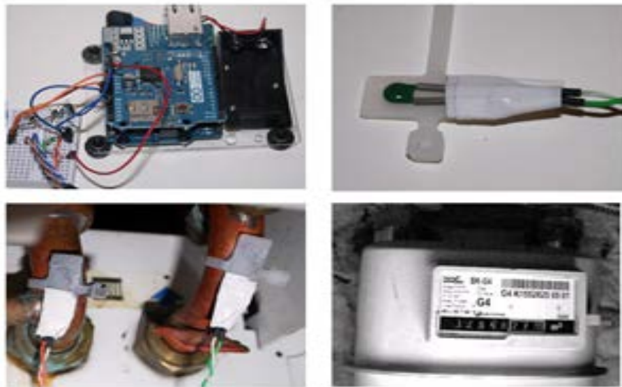
Figure 2. Prototype System including Arduino (top left), temperature sensors (top right), sensors affixed to pipes (bottom left), and feed from gas meter camera (bottom right).
