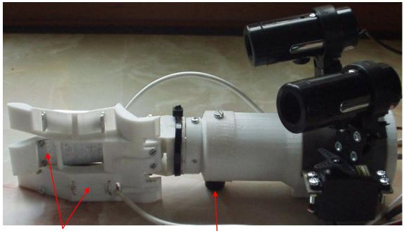
The two finger that house the force sensor electronics
