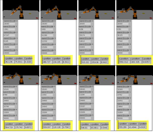
Table 5 Manipulator Maneauvres from Short Scan to Object Under Inspection
