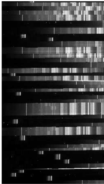
Figure 5.2: The flat fielded and bias subtracted science frame showing the first order spectra with sky lines and the zero'th order contamination.
