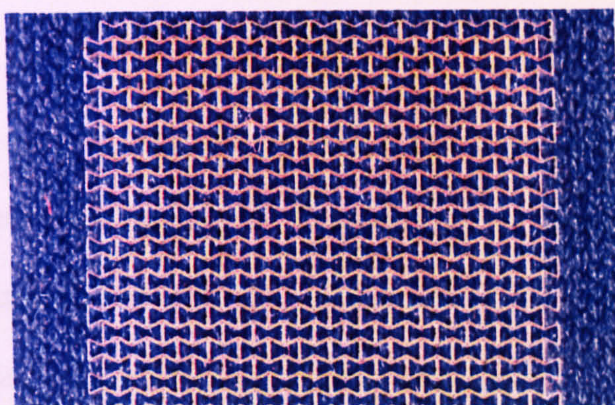
Fig. 4.2.6 Auxetic polymeric membrane formed by femtosecond laser ablation.
