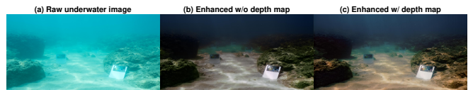
Fig. 6. Visual comparison on a sample from SQUID dataset [28], from left to right, shown raw underwater image, enhanced Image without and with depth map.
