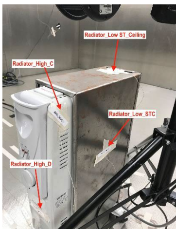
Radiator surface temperature sensors
