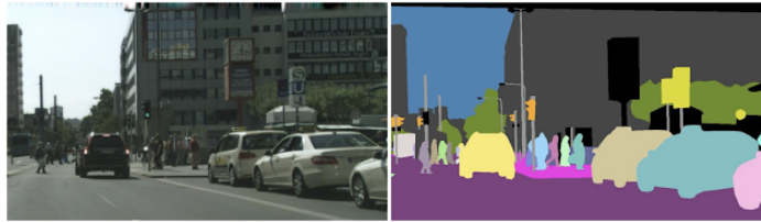
Fig. 17.6: Segmentation for object identification in a traffic image. Source: Cityscapes Dataset [19] https://www.cityscapes-dataset.com/ .
