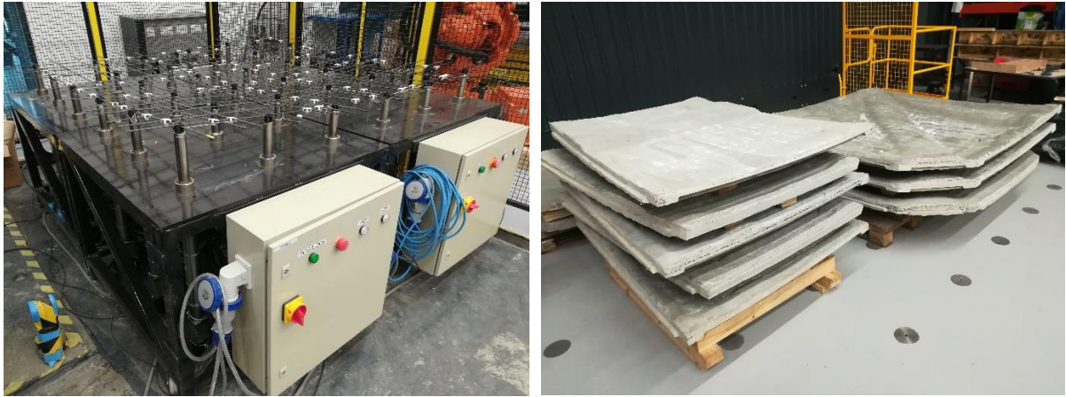
Figure 3 – Reconfigurable mould actuated by a set of vertical mechanically driven pins and connecting flexible formwork (left) and prefabricated segments ready to be transported and assembled (right). Photo credit: ©Robin Oval
