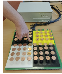
Fig 2: Photograph of 16-channel MIT instrument and 16-coil planar array with deformable membrane skin fitted, where a single membrane element of the skin is shown manually displaced or touched.
