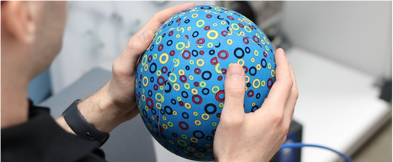
Figure 1: Our constructed shape-changing biofeedback-based pneumatic PAWS inflates and deflates in relation to captured inhalation and exhalation bio-signals.
