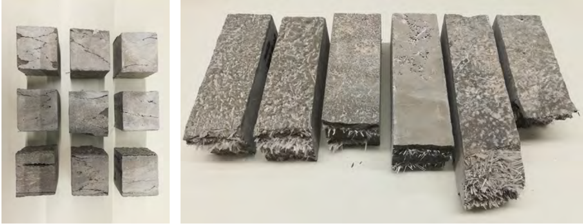
(a) Compression failure
