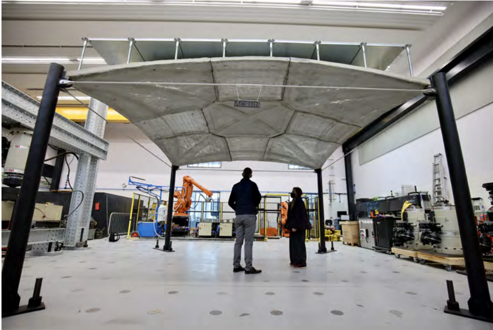
Figure 1: The OAK, ACORN’s demonstrator of a segmented ribbed concrete shell as a building floor for a circular economy of construction ©John Orr.
