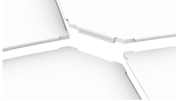
Figure 6: Exploded view of the half-joints acting as shear keys at the interfaces between segments.
