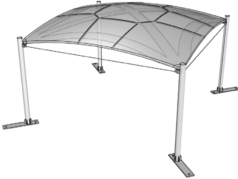
Figure 2: Render of the shell on columns, with tie-rods countering the thrust, after form finding, segmentation design, and connection detailing, including architectural, engineering, and construction requirements.
