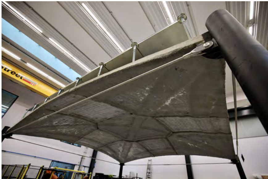
Figure 15: Shell standing once assembled on columns with a levelled floor ©John Orr.
