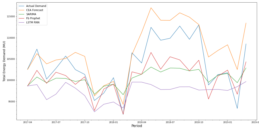
Figure 6: Visual comparison between SARIMA, LSTM RNN, Fb Prophet and CEA models for predicting monthly total energy demand
