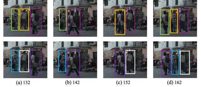
Fig. 5. Visualization of the qualitative results with tube re-assignment. The results are from frames 132, 142, 152, and 162 of sequence MOT17-01. Top row: The results without tube re-assignment make identity association with regression, resulting in ID switches when severe occlusions exist. Bottom row: With tube re-assignment, the motion cues are considered. Thus the identities are assigned correctly. (For interpretation of the references to color in this figure legend, the reader is referred to the web version of this article.)
