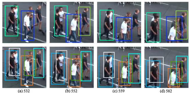
Fig. 7. Qualitative comparison results with the baseline and our method. The tracking results are obtained from frames 532, 552, 559, and 582 of test sequence MOT20-08, which is captured with frequent occlusions. Different box colors represent different identities. Top row: The tracking results of Tracktor. Bottom row: The results of our method. (For interpretation of the references to color in this figure legend, the reader is referred to the web version of this article.)
