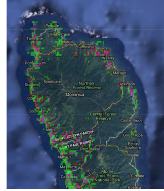
Figure 1: Heatmap of building damage proportion in Northern Dominica after hurricane Maria in 2017: less than 20% (green), 20% to 60% (magenta), greater than 60% (red).
