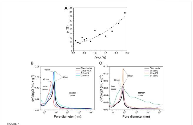
MIP results of the specimens at the curing age of 97 days (A) Development of capillary porosity  $\phi$  with the increasing fibre loading f (B) differential pore size distribution at lower fibre contents, CF0.005 vol%, CF0.2 vol%, and CF0.6 vol% as examples (C) differential pore size distribution at higher fibre contents, CF0.8 vol%, CF1.5 vol%, and CF2.4 vol% as examples.
