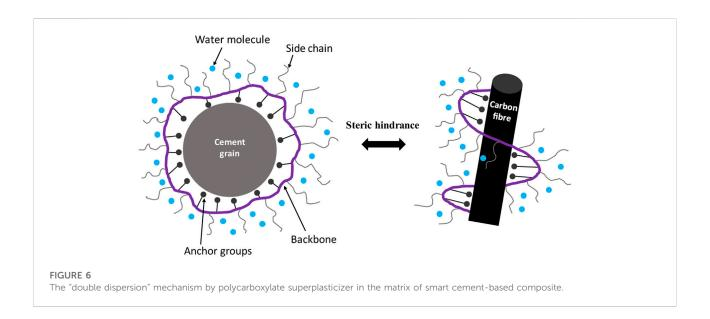
steric stabilization, and to create repulsion force *via* steric hindrance hence facilitating the dispersion of carbon fibres and cement grain (Figure 6).
