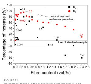
Percentage change in the mechanical performances  $R_c$  and  $R_f$  of smart cement-based composites at fibre contents 0–2.4 vol % relative to the plain mortar (marked as line of standard strength).
