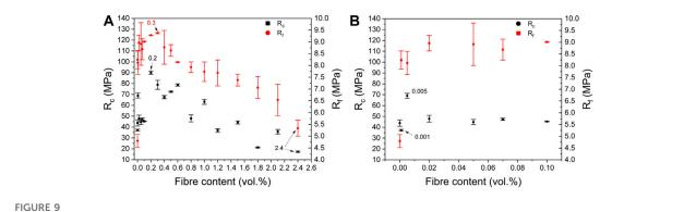
Arithmetic means and standard deviations of compressive strength  $R_c$  and flexural strength  $R_f$  for **(A)** smart cement-based composites with fibre contents 0–2.4 vol% **(B)** magnified plot for smart cement-based composites with near-zero fibre contents 0–0.1 vol%.
