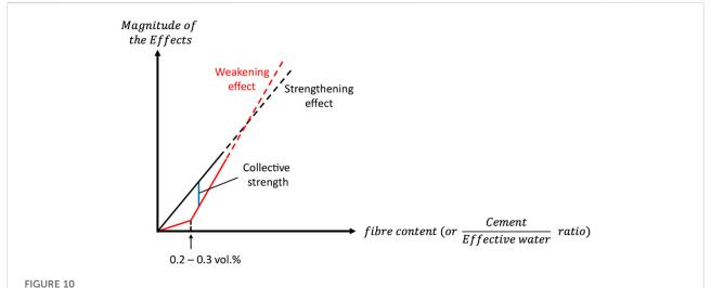
Schematic illustration for the development of the strengthening and weakening effects with the increasing fibre content (which is inversely proportional to the effective water/cement ratio). The collective strength can be calculated by subtracting the magnitude of the weakening effect from the strengthening effect.
