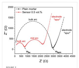
Nyquist plot of smart cement-based composite (CF0.5 vol% as an example) and plain mortar both at the age of 97 days and water-saturated condition,  $\omega_{\rm bs}$  refers to the angular frequency for the bulk resistance of the smart cement-based composite,  $\omega_{\rm bpm}$  refers to the angular frequency for the bulk resistance of the
