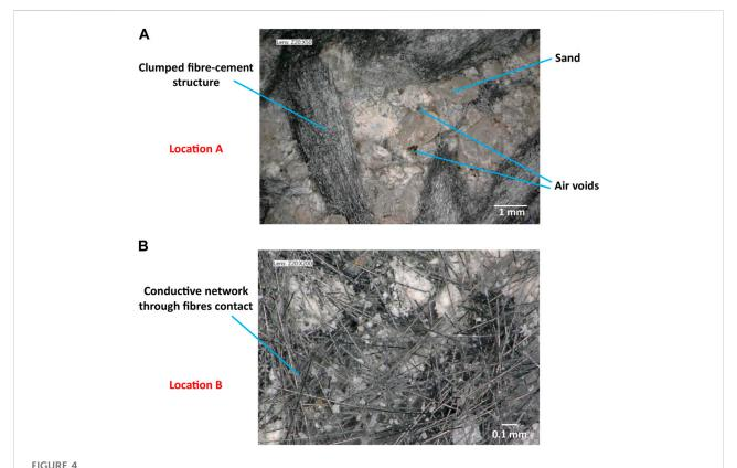
Digital microscope investigation on the fracture surface of CF2.4 vol% (A) location A where the fibres were clumped, the sands were poorly bonded, and the mortar matrix showed poor homogeneity (B) location B where the fibres were uniformly dispersed but still the mortar matrix showed poor homogeneity.
