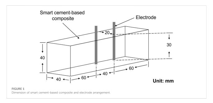
of blending for improved matrix homogenization. The fibres were initially dispersed into the polycarboxylate solution before blending with the cement powder and the standard sand. The physical properties of smart cement-based composite can be influenced by the manufacturing process, therefore the manufacturing process is introduced in detail:
