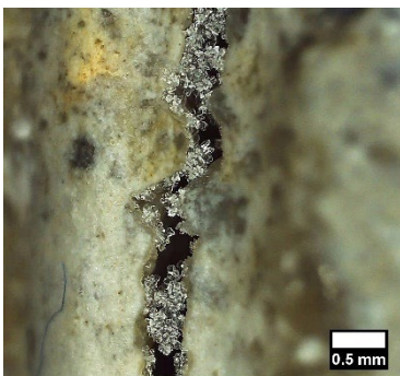
Fig. 9: Digital microscope image of a crack in a mortar specimen (H_C_SD) showing newly formed CaCO 3 crystals after seven days of healing.
