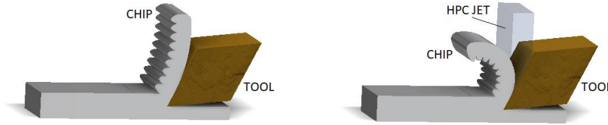
Fig. 7 - Effect of the hydraulic wedge on chip curling [110, 111]
