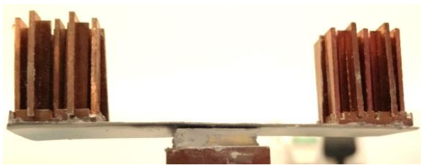
Figure 16. TEG-heatsink assembly experimental set-up and results (a) without PGS, (b) with PGS on top of the copper sheet and (c) with PGS on bottom of the copper sheet.
