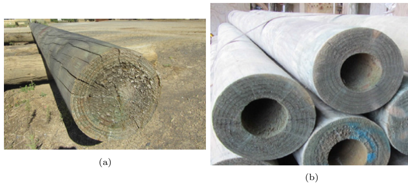
Figure 12: 12a) Whole timbers exhibit longitudinal cracking when dried. 12b) Cored timbers show less longitudinal cracking due to reduced internal drying stresses. Photographs courtesy of TTT Products Ltd. and Mark L. Batchelar.
