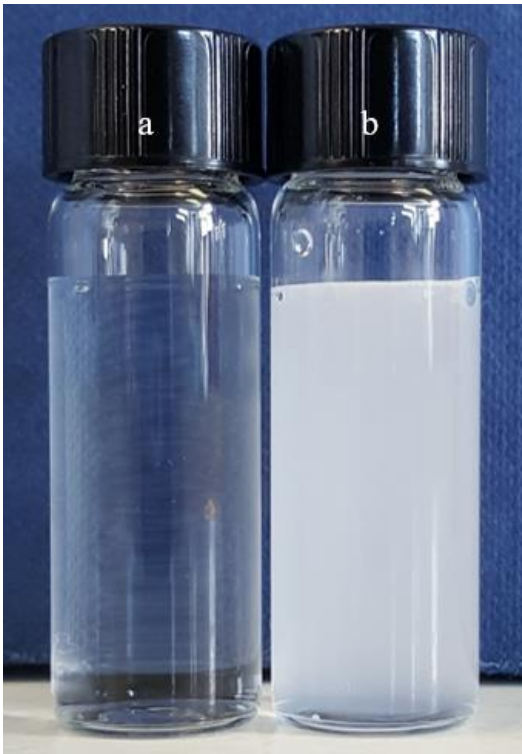
Fig. S5. Oil in water emulsion (a) the permeate, (b) the feed before ultrafiltration process
