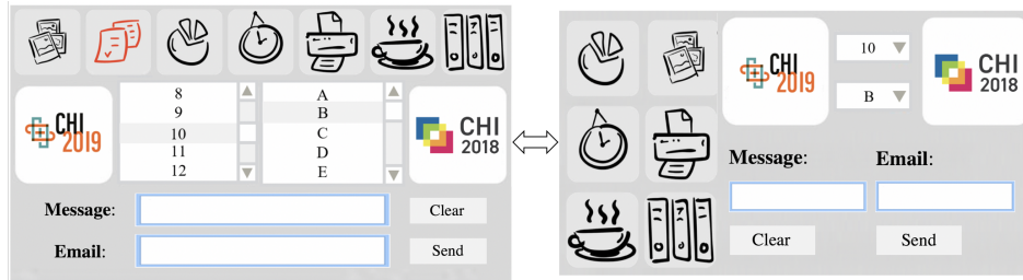
Figure 9: A more complex example combining the alternative position pattern for the toolbar at the top and the widgets at the bottom, the balanced flow and optional layout patterns for the toolbar, and the alternative widgets pattern for the list boxes.
