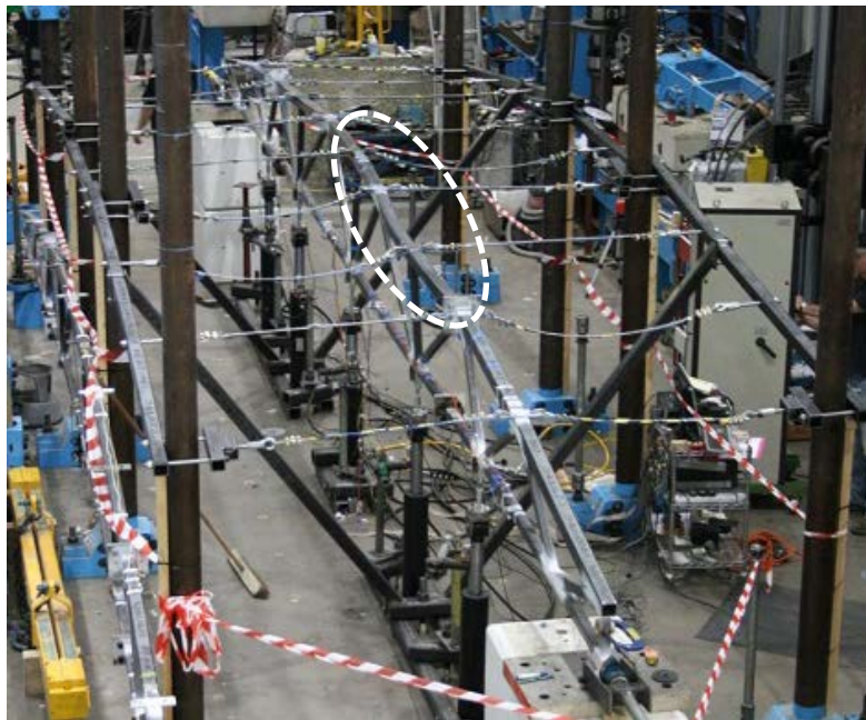
(b) Out-of-plane buckling of top chord of Truss 3
