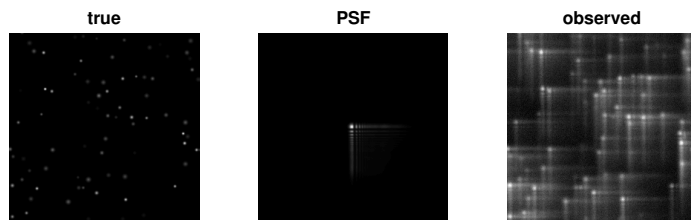
FIG. 4. Experiment 1: Image deblurring example. Here we show the true image, the point spread function (PSF), and the observed blurred and noisy image. The size of the images is 256 \times 256 pixels.
